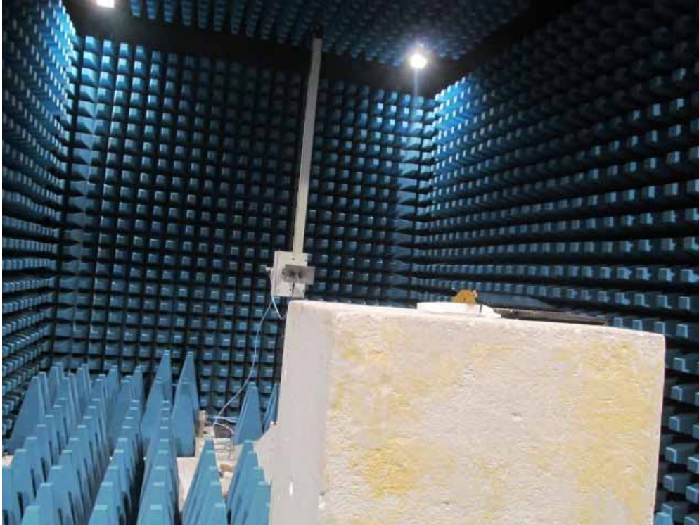
Description: Receive Spurious Emissions Test Setup for Above 1GHz
